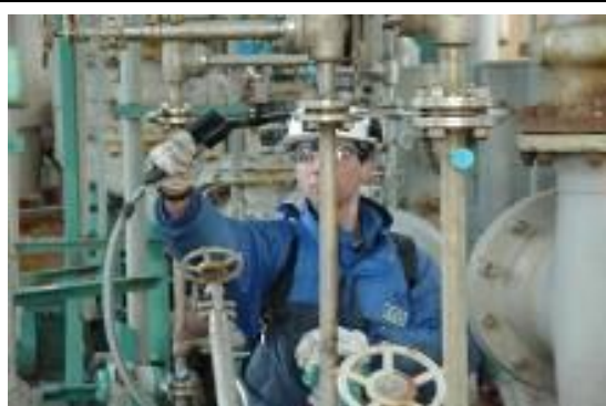
Figure 3.37: Leak concentration measurement
