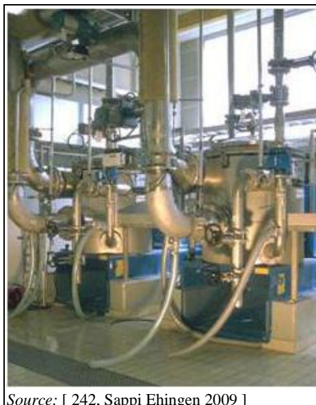
Figure 4.7: Pressure screens for final screening
