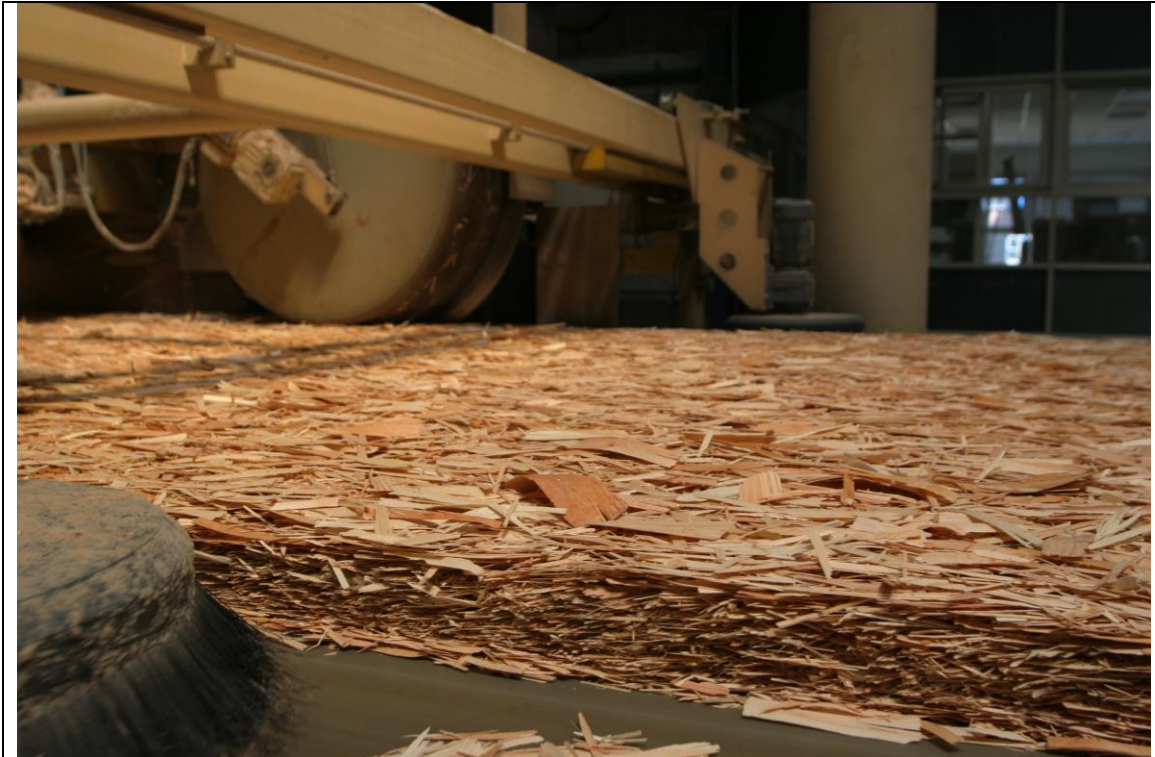
Figure 2.8: OSB mat after forming and trimming
