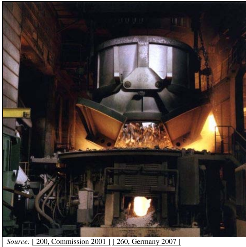
Figure 8.2: Electric arc furnace charging
